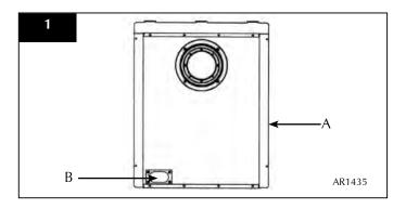
5.2 Gas pipe entry must come through the rear right-hand side of the box. The rubber seal must be cut using a sharp knife to allow the isolating elbow to pass through it.
